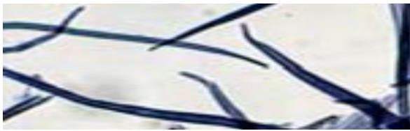
Figure 2: Fiber image of Oil Palm EFB on projection microscope
